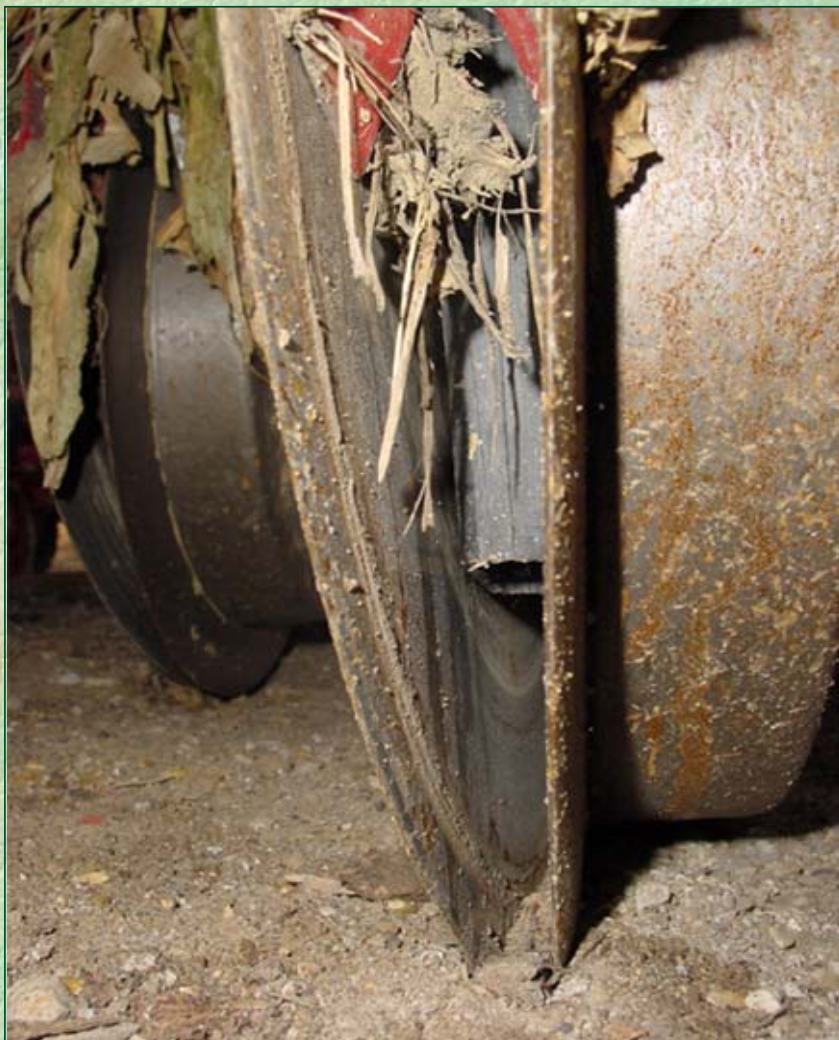
A double disk cuts the mulch for sowing
