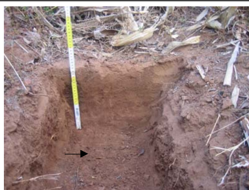
Fig.5: Blantyre, Malawi – soil profile, compacted in 15 cm depth and deeper
